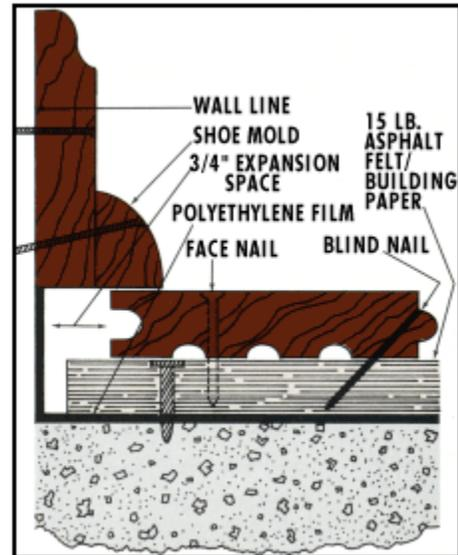
Fig. 1. Plywood-on-slab method of installing strip oak flooring
