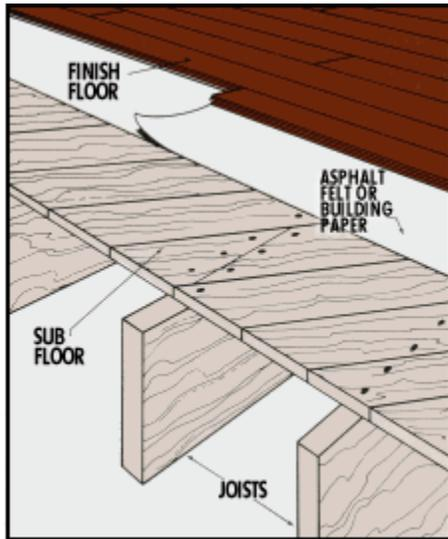
Fig. 4. Wood joist construction using square-edge board subfloor.
