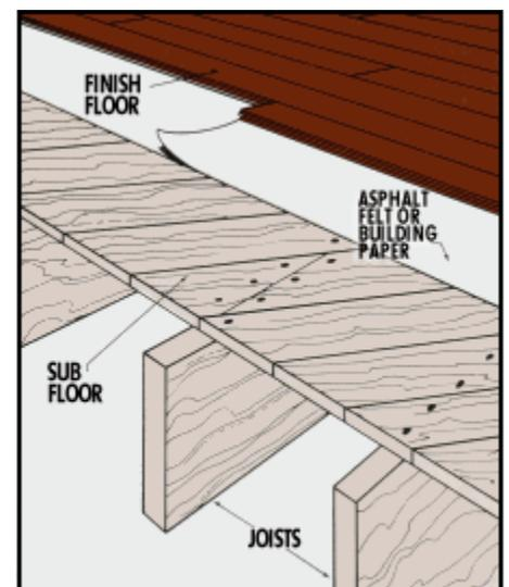
Fig. 4. Wood joist construction using square-edge board subfloor.
