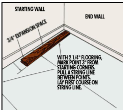
Fig. 5. Establishing starter line for nailing first strip.
